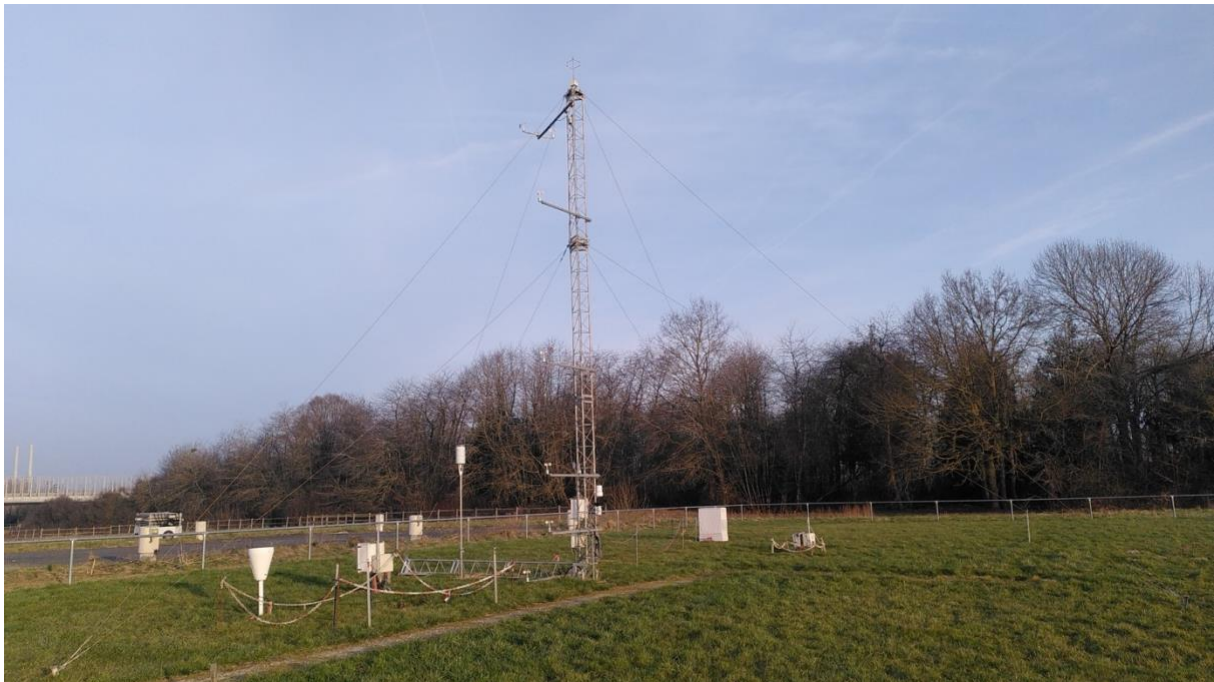
Figure 6 SIRTA's state-of-the-art meteorological station measuring several variables, such as air temperature and wind speed
