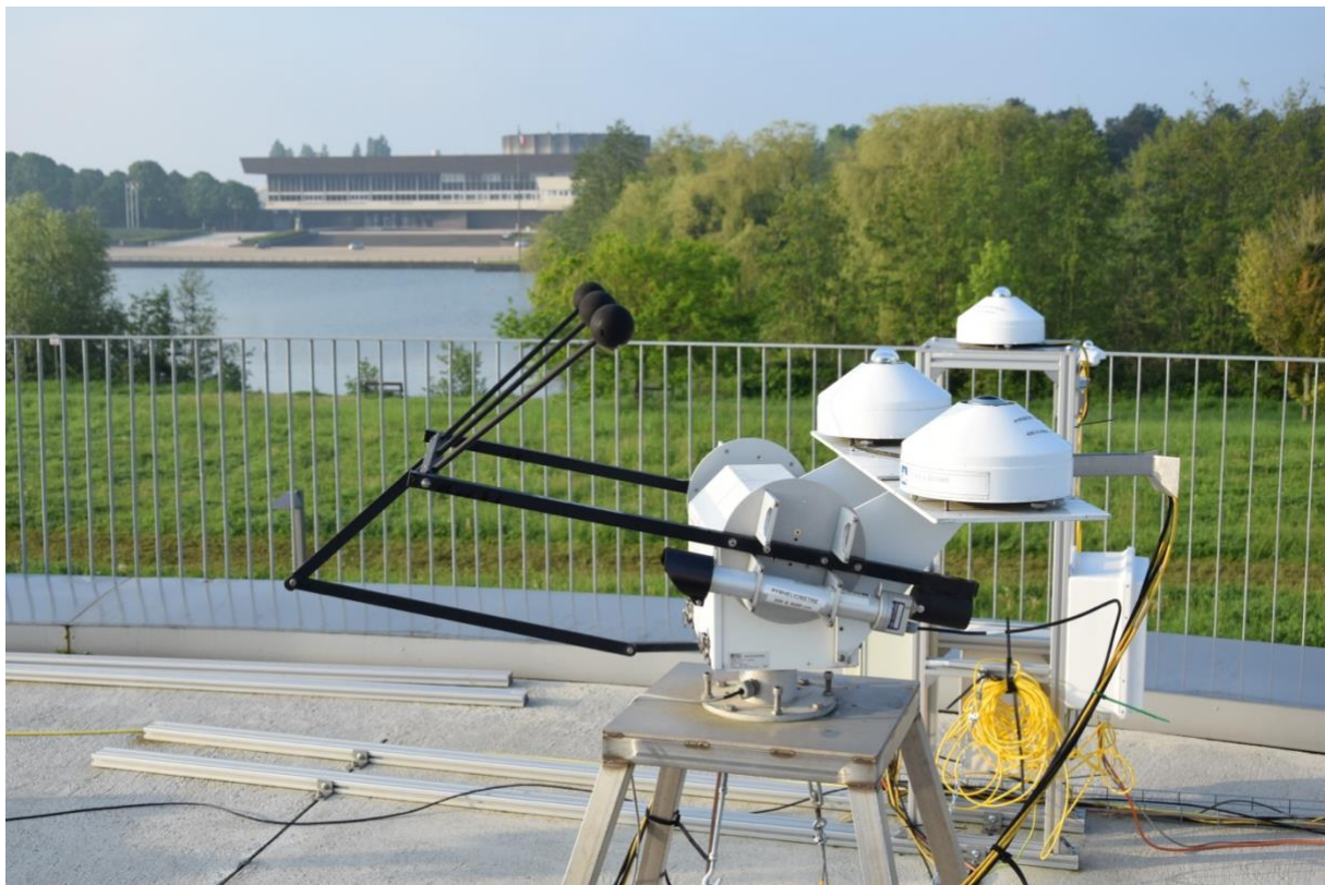
Figure 5 SIRTA's roof-top radiative installation measuring solar global, direct and diffuse irradiance
