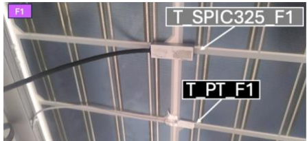
Figure 11 Top : Layout of reference cells and the PV module temperature locations. Photos: views of all sensors
