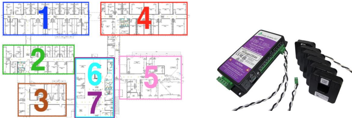
Figure 10 (left) Location of the 7 electric Zones of the Drahi-X buildings for which consumption measurements exist since July 2016 (right) photo of the type of egauge devices installed ( www.egauge.net )
