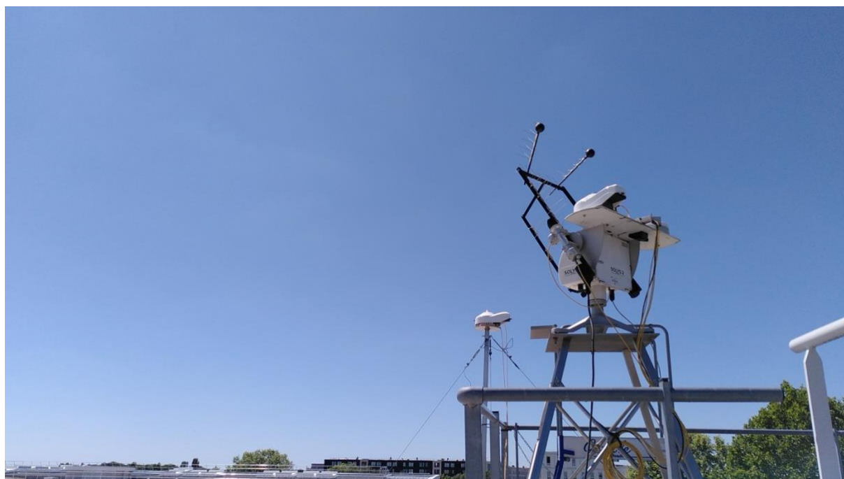
Figure 21 BSRN (baseline surface radiation network) installation at SIRTA with Global, direct, diffuse solar irradiance as well as infrared irradiance measurements
